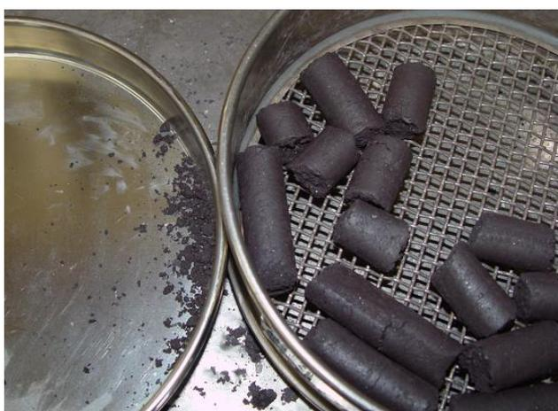
Figure 9 Drop testing of experimental BREX results (left – fines generated; right – dropped samples)
