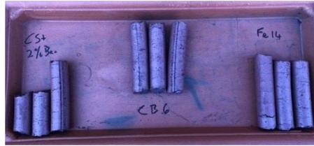
Figure 5 BREX after 5 minutes exposure at T = 900 °C
