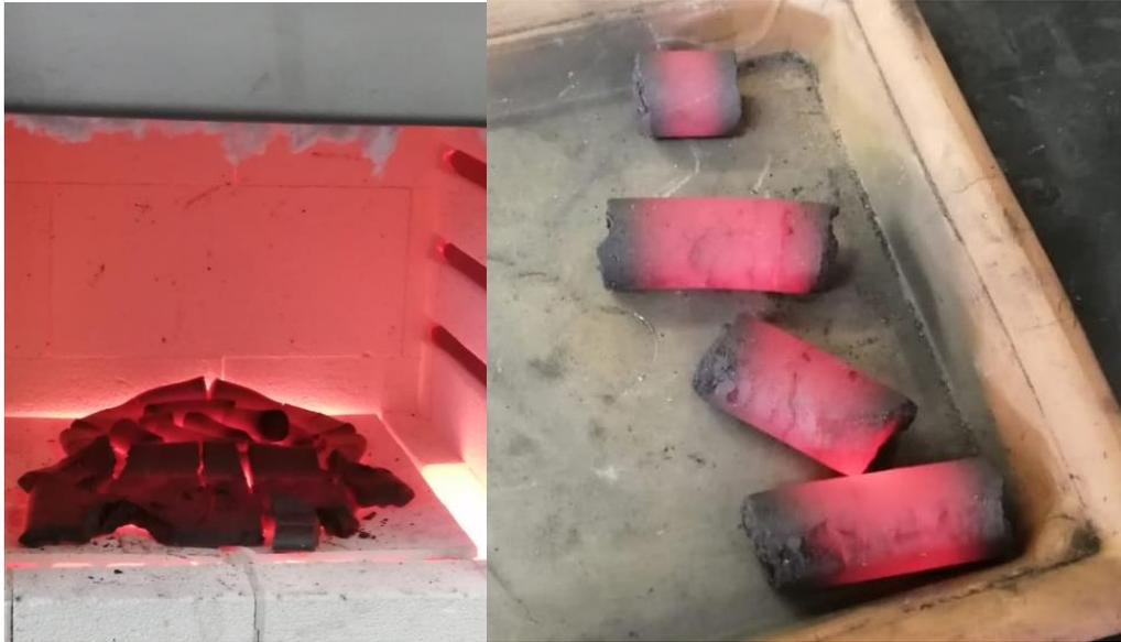
Figure 12 Appearance of the BREX during thermal stability testing (left) and after extraction from the furnace
