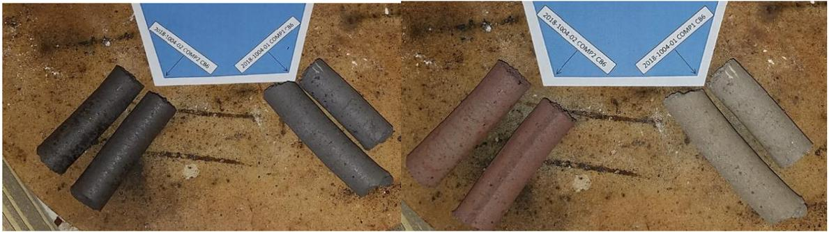
Figure 10 Appearance of experimental BREX (left – raw; right – partially reduced) after heating to 900°C
