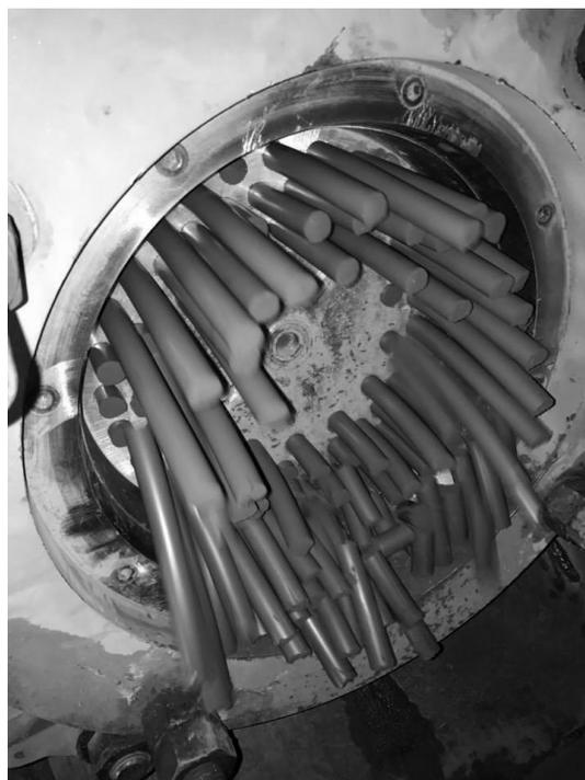
Fig. 8.25 Industrial production of chromium-based brex at Aktobe Ferroalloy Plant
